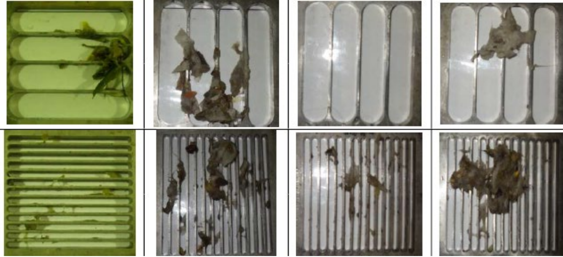
Figure 4 Example of test results for 25 mm (1") slotted coarse screen followed by 6 mm (1/4") slotted fine screen
